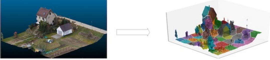
Figure 4.2: Clustering results of the 3D mesh faces. Each color represents a distinct cluster, which serves as a local patch for input into the model.
