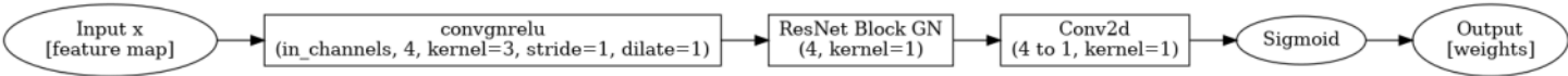
Figure 4.6: Layout of the Inter-view Adaptive Aggregation Module to combine features of different viewpoints.
