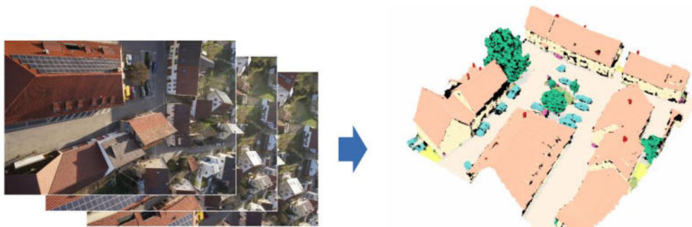
Figure 1: Example of a multi-view stereo reconstruction. Multiple images of the same urban scene taken from different viewpoints under slightly varying conditions serve as input to the multi-view stereo procedure to be developed to reconstruct the 3D geometry of this scene.
