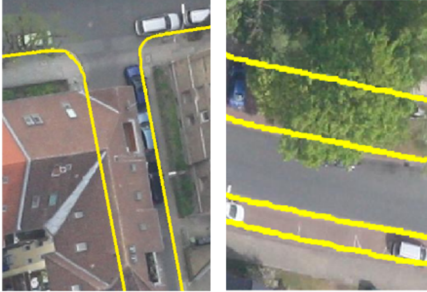
Figure 12: Areas without curbstone annotations (marked with the yellow lines), curbstones occluded by buildings and tree branches (Tian et al. (2023))
