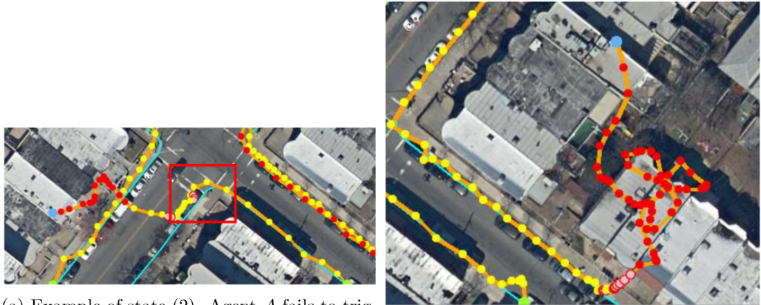
(a) Example of state (2). Agent A fails to trigger a stop action or make corrections when it generates incorrect vertices (in the red rectangle). Then an obvious incorrect curb instance is obtained. (b) Example of state (2) and state (1). Agent A fails to stop when it is close to the end vertex, turns in the wrong direction, and generates many meaningless vertices.
