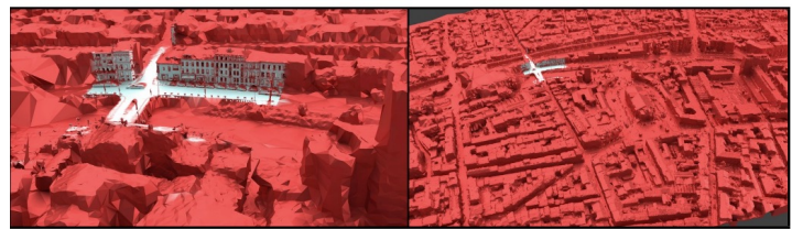
Integrating data in the same geometric reference frame Space-triangulation and aerial-triangulation (left) Registration of mobile mapping lidar on 3D city data (right)
