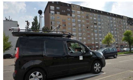
Mobile mapping system Stereopolis 3.0. IGN ©
